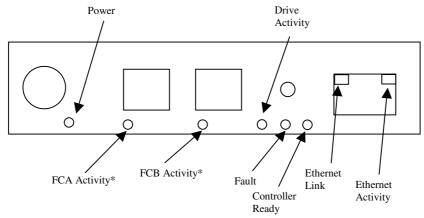
\*Note: Even though a cable may be connected, the indicator activity LED's will only illuminate when there is activity on that channel.
